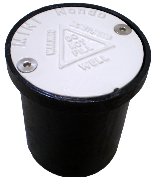
Mini Nondo Well Cover: Small cover ideal for soil vapour installations. Only 150mm OD, 124mm ID, 150mm cast iron skirt, Flush mount, bolt down lid, oring sealed.
